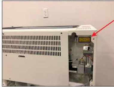
CABINET REAR RIGHT INSIDE OPTICS ADJUSTMENT ACCESS PANEL
