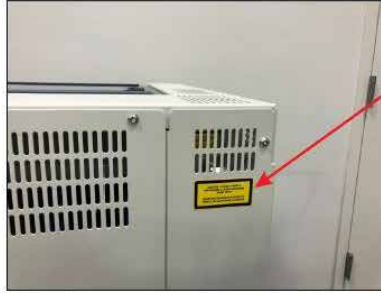
CABINET REAR RIGHT OPTICS ADJUSTMENT ACCESS PANEL
