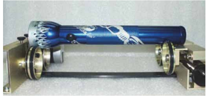
Correct Setup: The flashlight is horizontal to the X-Beam
